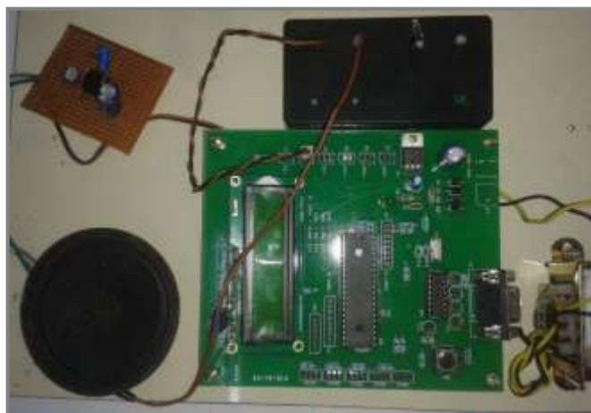
Figure 4: Li-Fi Transmitter and Receiver Circuits
