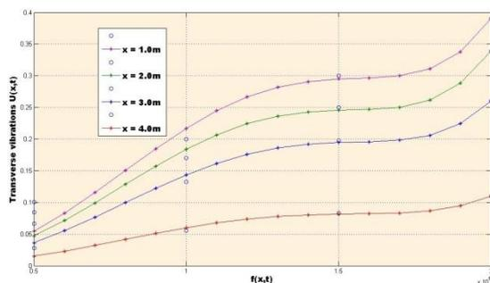
Figure 2b: Graph of Transverse Vibrations against External Force at Varying Bridge Length
