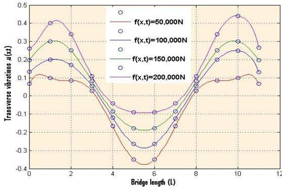
Figure 2a: Graph of Transverse Vibrations against Bridge Length at Varying External Force
